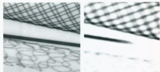
Blurry image of stents on the right was taken using conventional X-ray image intensifier technology; clear image on the left was taken using the high-resolution region-of-interest microangiographic digital detector being developed at UB. Each photograph shows two stents separated by a 26-gauge needle. The stent above the needle is a self-expanding Wallstent with 80 micron stainless steel wire; the stent below the needle is a balloon expandable MultiLink stent with 50 micron wire.
